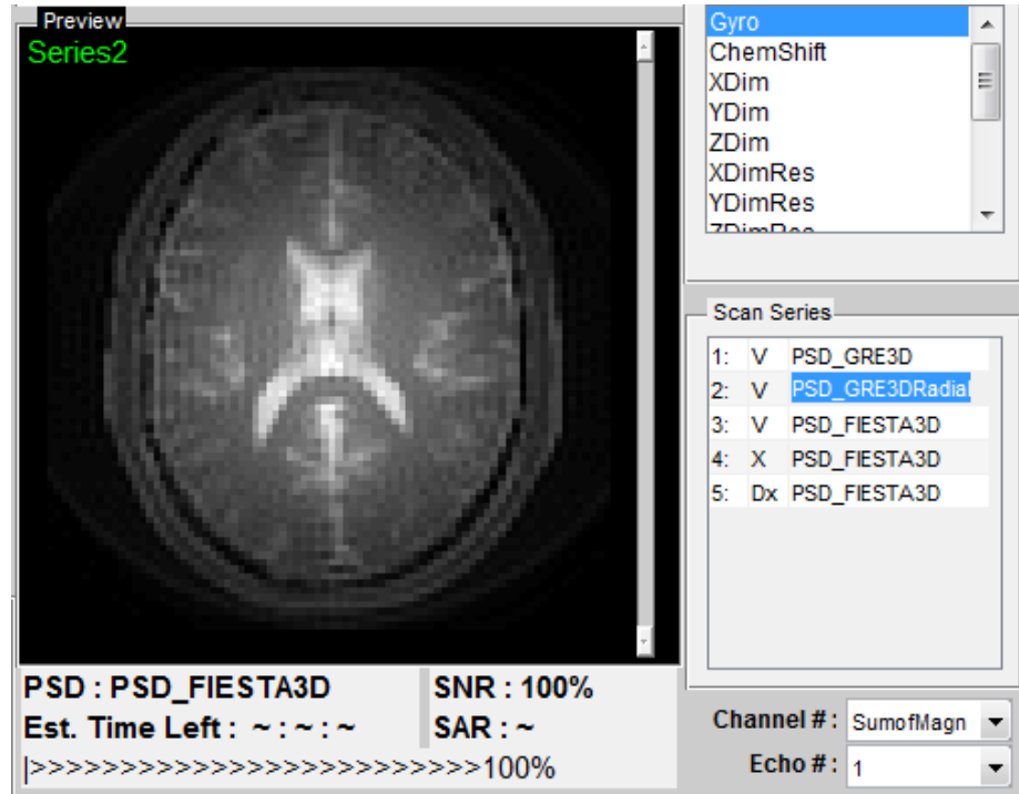
Figure 4.1: The Preview of A Simulated Image. The preview is one slice of simulated image using gradient echo sequence with radial readout and reconstructed without deapodization.
