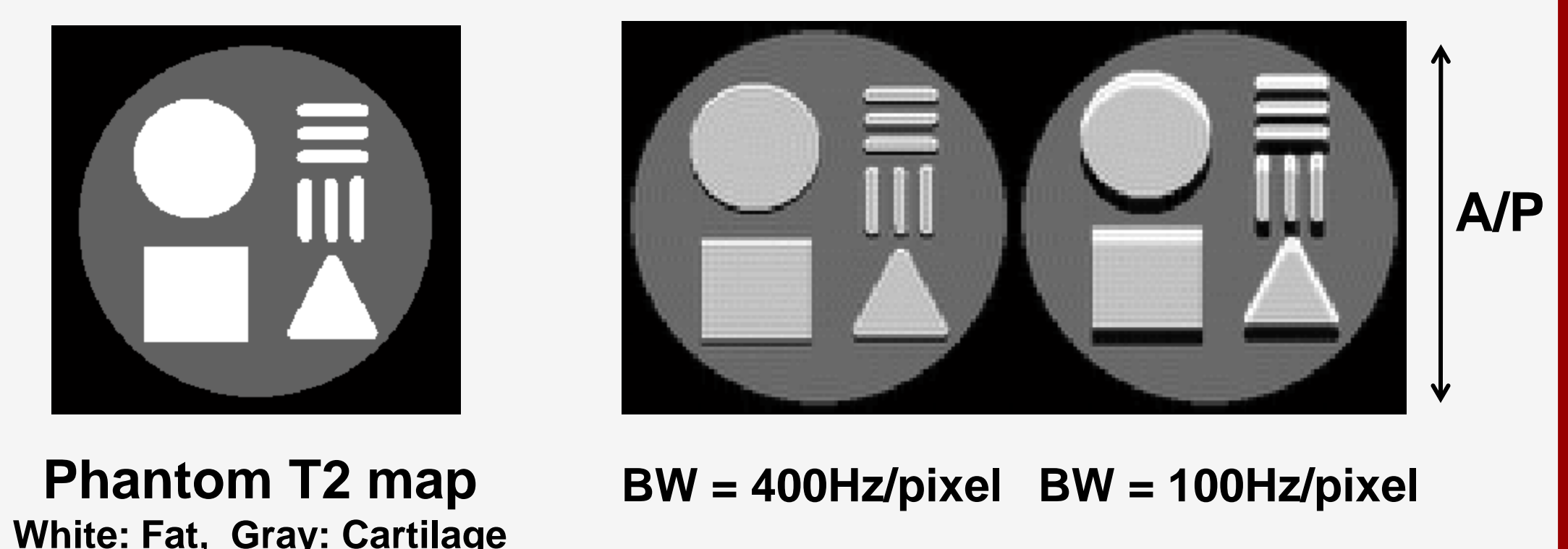
Figure 7. Simulated 3D gradient echo image at 3.0T using cartilage-fat phantom showing water fat chemical shift at different readout bandwidth. The phantom size is 256x256x32x2, simulated in-plane matrix size is 100x100, TR/TE = 10s/50ms, Axial plane, A/P readout.
